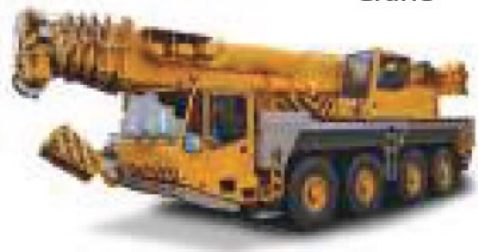
All Terrain Crane
